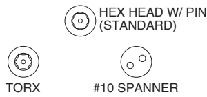
TAMPER RESISTANT SCREW HEADS OPTION SUFFIX- T3
