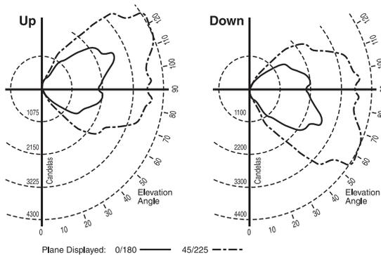
*Unique reflector system maximizes light where you need it most, rotates 30° up or down.*
